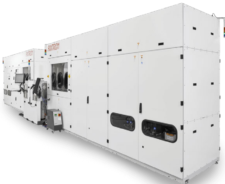
Example picture of two AIXTRON G5+ process modules connected with a cassette to cassette handling system
