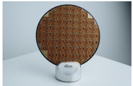
Fully processed 200mm GaN-on-Si wafer with power HEMT devices
