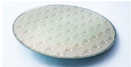
200 mm GaN-on-QST ® , with processed trench gate MOSFET devices
